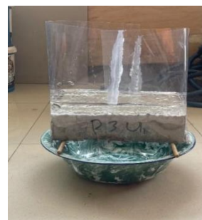
Gambar 3. Uji infiltrasi paving block
